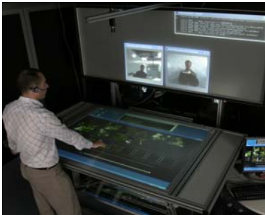
The ViCAT table, with a shared multi-cursor video editing application displayed on the horizontal screen ('task space' [1]) and remote collaborators showing on the vertical screen ('person space' [1]).
